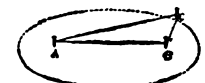
To Draw an Ellipse. A, B, fixed points; C, moving point; A, B, C, elliptical.
