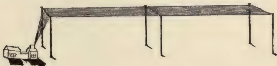
FIG. 11.—Aerial conductor of Mr. Marconi's Transatlantic Station at Clifden, Ireland. For short distances the fan-shaped portion would be sufficient. The horizontal wires are added to give greater power for long distances.
