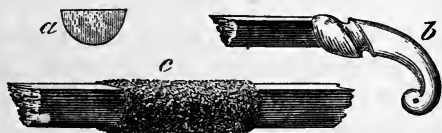
a , Section of bow; b , end of bow, showing nock; c , handle of bow.
