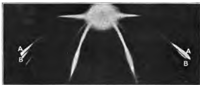
FIG. 17. Parabolas obtained in positive ray analysis by J. J. Thomson. Neon gave two parabolas, A and B. (A retouched photograph of the illustration in the original memoir.)
