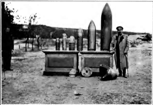
UNEXPLODED GERMAN SHELLS. THE LARGEST IS FROM THE 16-INCH SIEGE GUN, THE NEXT LARGEST FROM THE 11-INCH FIELD HOWITZER
