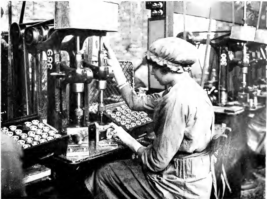
DRILLING SAFETY-PIN HOLE IN FUSE
