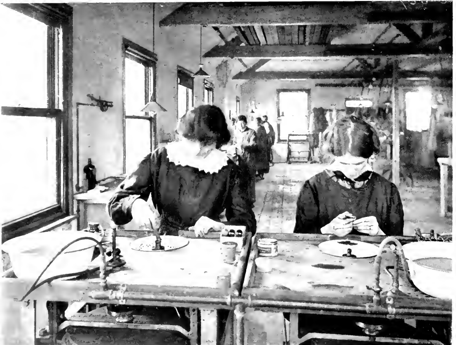
TREADLE POLISHING-MACHINES, FOR SMOOTHING LENSES
