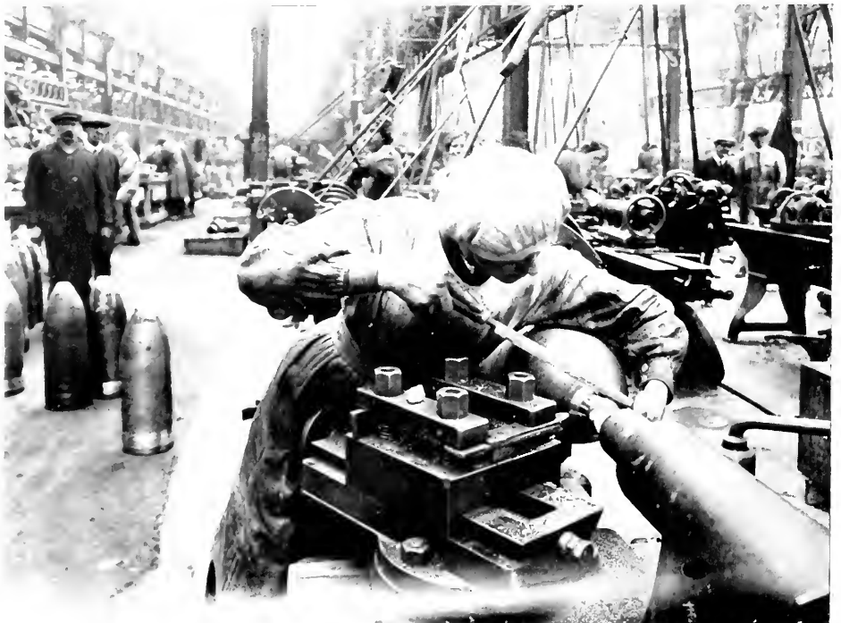
TURNING THE OUTSIDE AND FORMING THE NOSE-END OF A 9.2-INCH HIGH-EXPLOSIVE SHELL
