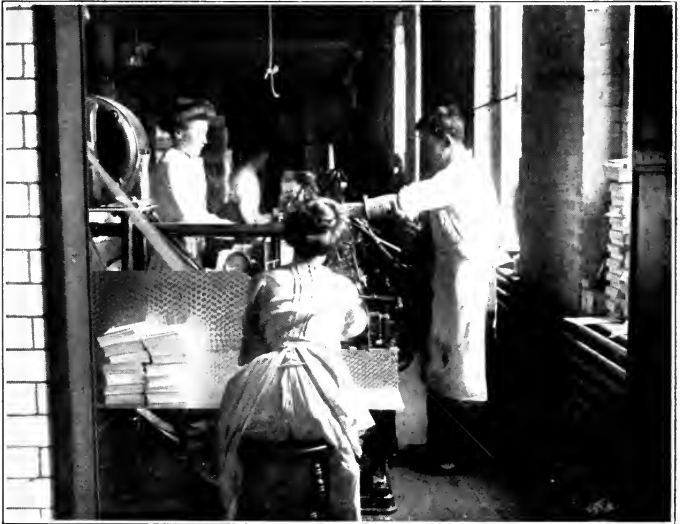
GATHERING MACHINE (Man operating and women filling the boxes and taking out the gathered books)
