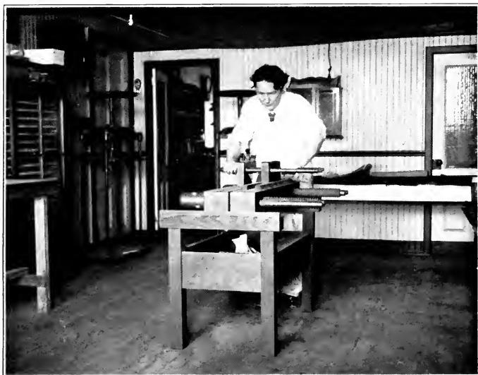
PRESS AND PLOW MACHINE (The primitive way of plowing or cutting)
