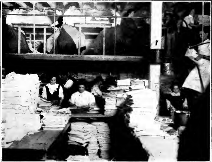
FOLDING AND GATHERING (Hand folders on platform; machine folders and hand gatherers below)
