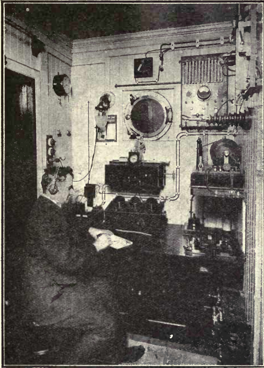
FIG. 41.—Arrangement of receiving apparatus in the ship's wireless cabin.
