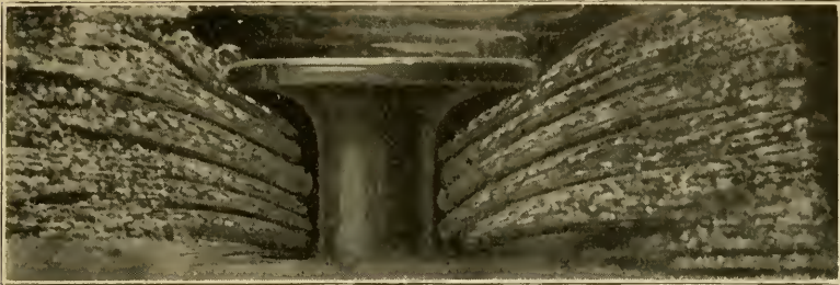
FIG. 19—Injury to wood fiber resulting from overdriving nails.
