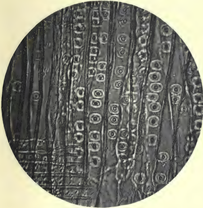
FIG. 9.—Longitudinal radial section of Pinus Sylvestris timber showing well-developed bordered pits upon the walls of the tracheids. At right angles to the tracheids is a medullary ray.
