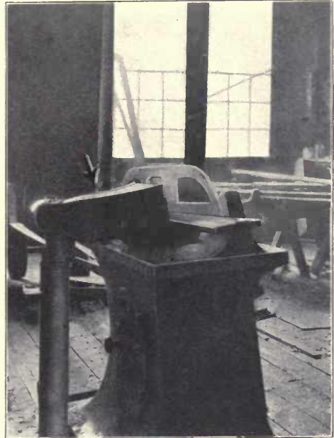
Fig. 79. Blower Hood for Panel Raiser.
