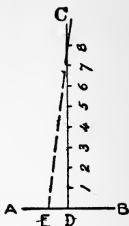
Fig. 316.—How to obtain Correct Angles for Dove-tail Template.
