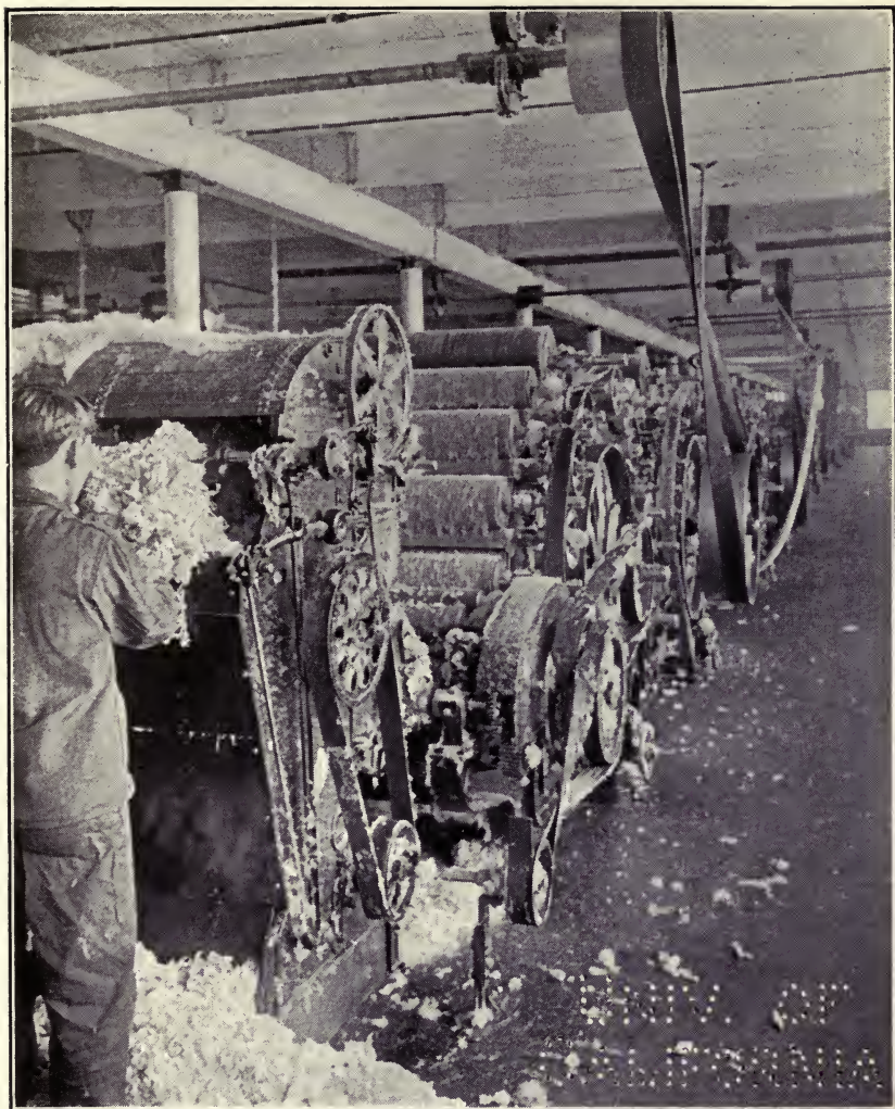
HERE IS SHOWN A SERIES OF CARDING MACHINES. WOOL IS BEING FED INTO THE NEAREST ONE, TO BE STRAIGHTENED OUT BY THOUSANDS OF SMALL TEETH ON REVOLVING DRUMS,
