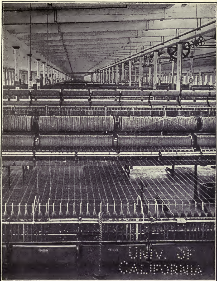
THIS PICTURE SHOWS PART OF A MULE SPINNING ROOM. THE PART OF THE MACHINE IN THE FOREGROUND MOVES BACK AND FORTH, DRAWING OUT AND TWISTING THE YARN.
