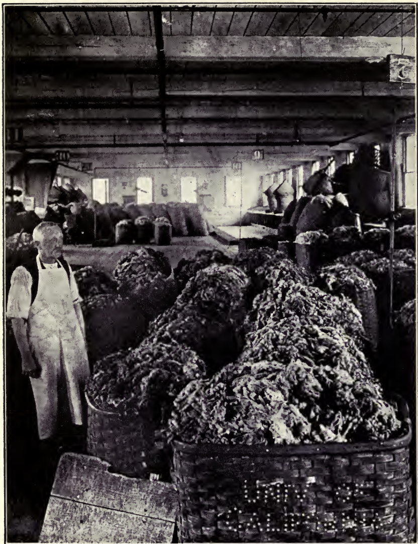
THIS IS HOW WOOL LOOKS WHEN RECEIVED AT THE MILL. IT COMES IN BAGS IN WHICH THE FLEECEES ARE TIED TOGETHER, WAITING TO BE SORTED INTO THEIR VARIOUS QUALITIES
