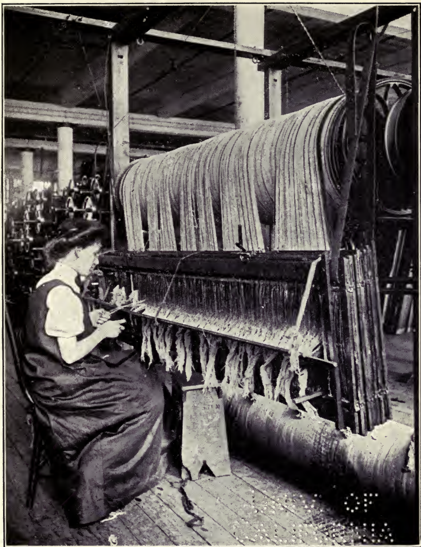
DRAWING WARP THREADS THROUGH THE HEDDLES IN THE HARNESSSES, WHICH CONTROL THE APPEARANCE OF THE WEAVE, AS THEY MOVE UP AND DOWN ACCORDING TO THE PATTERN
