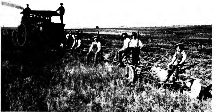
Twenty-four disc, steam plow, owned by Wm. Morris, Graham county. (4 rigs in county.) Cuts 4-inch sod, 16 feet to swath, turns 40 acres per day, and consumes 1½ tons of coal.
