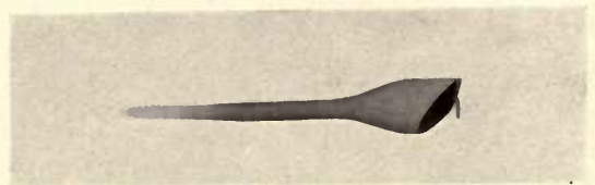
Fig. 12. Roentgenogram of Target of Tube in which Cathode is placed Very Close to Anode
