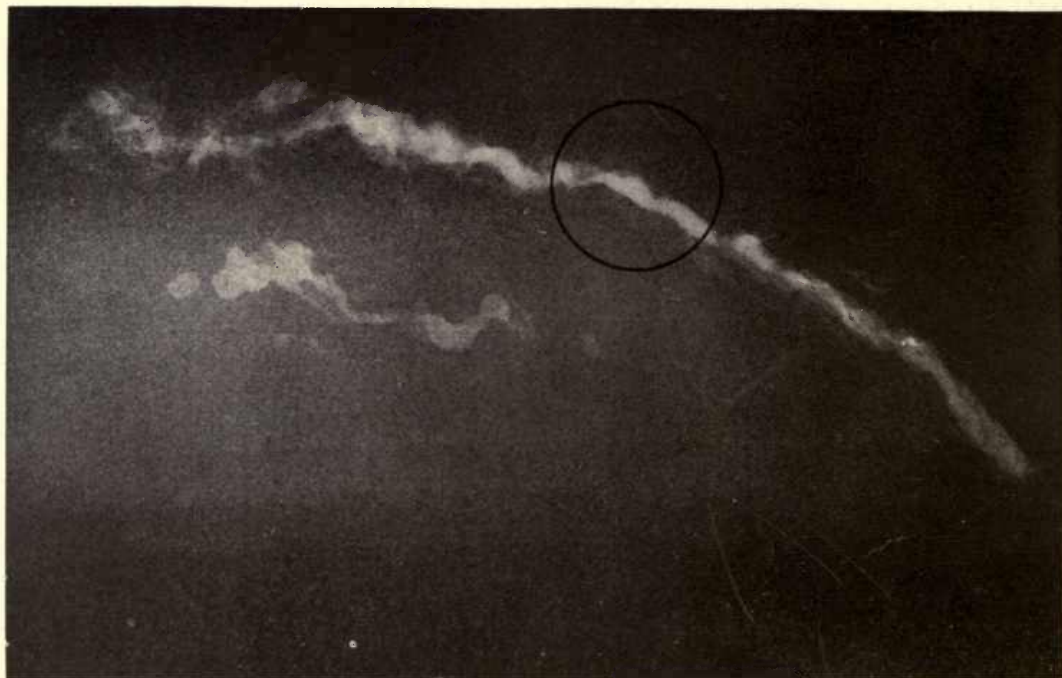
Fig. 1. Radiograph of a Steel Casting Showing Flaw Within Casting. The Circle Shows where a Piece was Later Punched Out
