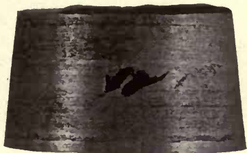
Fig. 2. Ordinary Photograph of One Edge of the Punching from the Plate Shown in Fig. 2. Note Flaw
