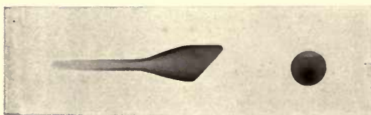
Fig. 17. Right, Roentgenogram of Target of Tube shown in Fig. 16; Left, Broadside View of Target for Comparison
