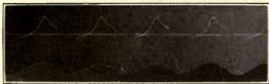
Fig. 13. W. & B. Transformer. Tube load: 100 M. A., 41 K Useful voltage above zero line and inverse voltage below
