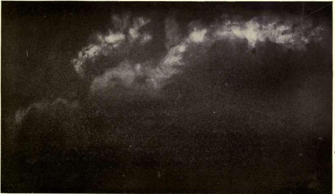
Fig. 8. A Radiograph of a Steel Casting Revealing a Flaw in the Interior of the Plate
