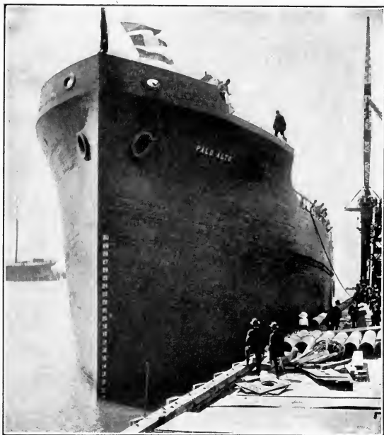
THE "PALO ALTO," FIRST CONCRETE SHIP OF ITS SIZE; IT IS OF 7,500 DEAD-WEIGHT-TON CAPACITY
