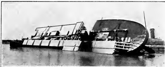
TURNING THE AFTER HALF OF THE "CHARLES R. VAN HISE" ON THE SIDE FOR TOWING THROUGH THE WELAND LOCKS FROM LAKE ERIE TO LAKE ONTARIO
