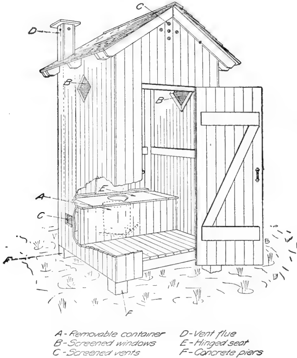
FIG. 28.—Outdoor, dry-earth, removable-container privy. Durable construction, well ventilated, and screened. With proper care is sanitary and unobjectionable.
