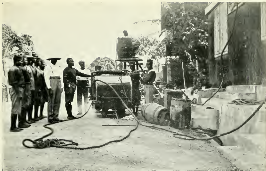
FIG. 54.—Generating the Sulphur in the Clayton Apparatus. Secondee, 1910.
