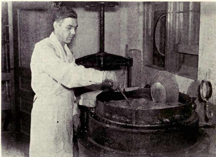
This is a steam-jacketed lard rendering kettle in use. Operator stirs lard almost constantly, breaking the lumps, until it is melted and starting to cook.
