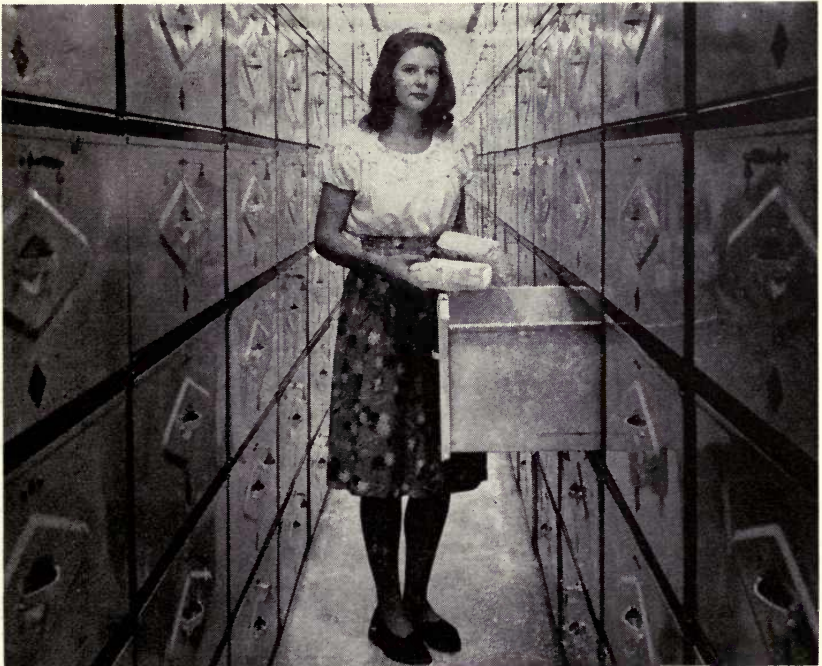
Minimum space for aisles is 34 inches. This permits drawers on opposite tiers of lockers to open fully. A better width is 36 inches.
