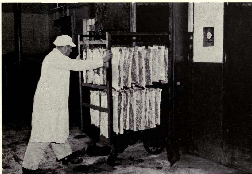
Wagon-racks are available which save much handling during the smoking process.
