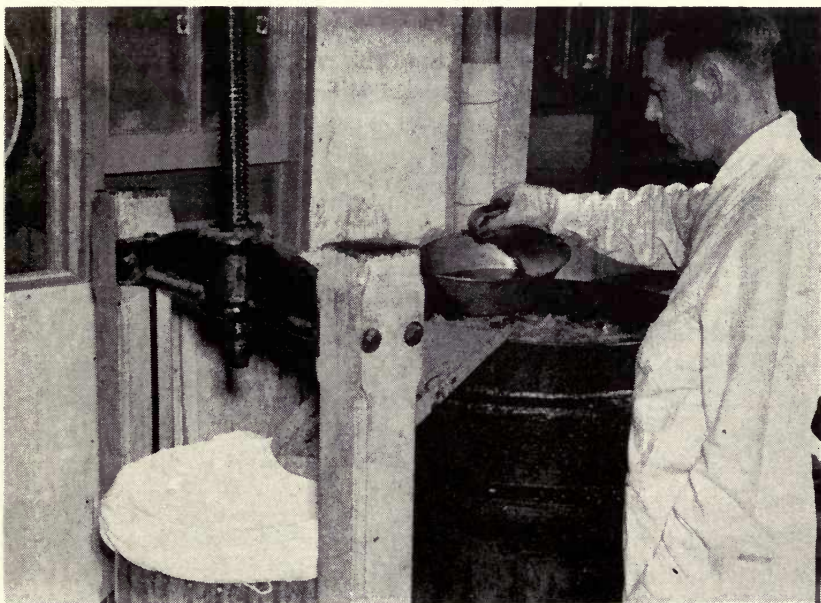
After the cooked lard is scooped from the kettle and strained through muslin into the lard press, cracklings are squeezed through the press.
