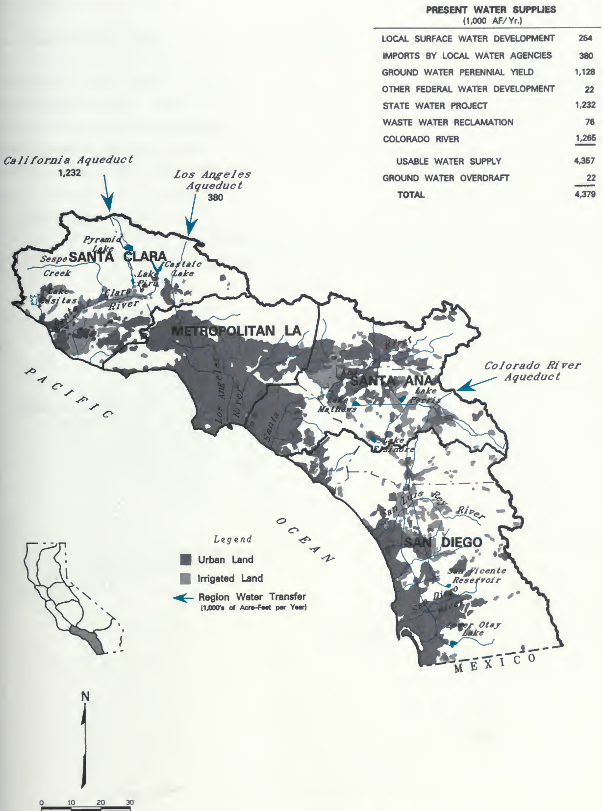
Figure SC-1. South Coast Region Land Use, Imports, Exports, and Water Supplies
