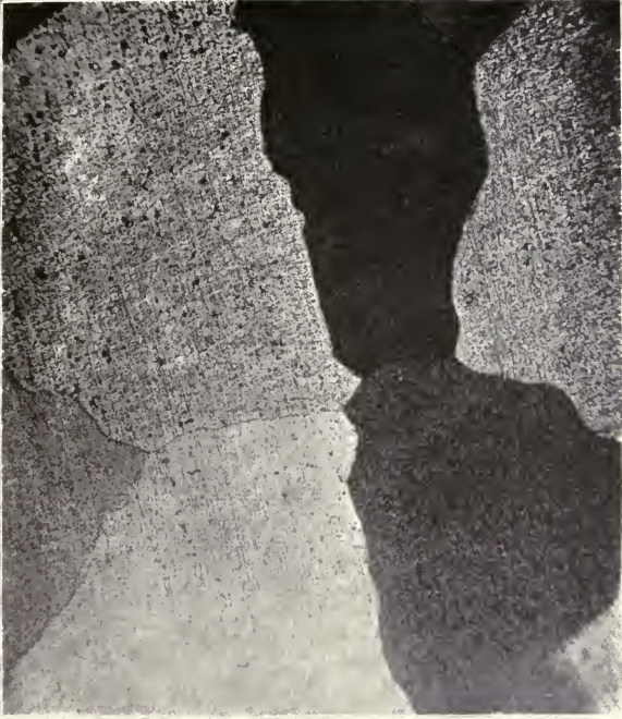
Brass (70 % copper, 30 % zinc) after annealing for one hour at 750° C.; showing crystalline structure. Magnified 80 diameters. Etched with 10 % solution of ammonium persulphate.
