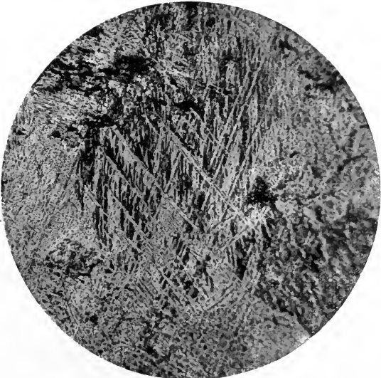
Photomicrograph of cast zinc (showing twinning). Magnified 100 diameters
