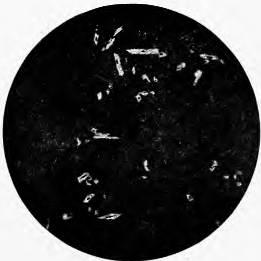
Photomicrograph of cast zinc with 3% of lead. Magnified 100 diameters.
