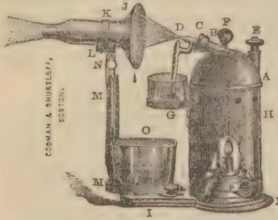
The waste-cup, medicament-cup, and lamp are held in their places in such a manner that they cannot fall out when the apparatus is carried or used over a bed or otherwise.
