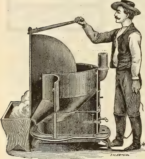
Showing Dumping Process.
