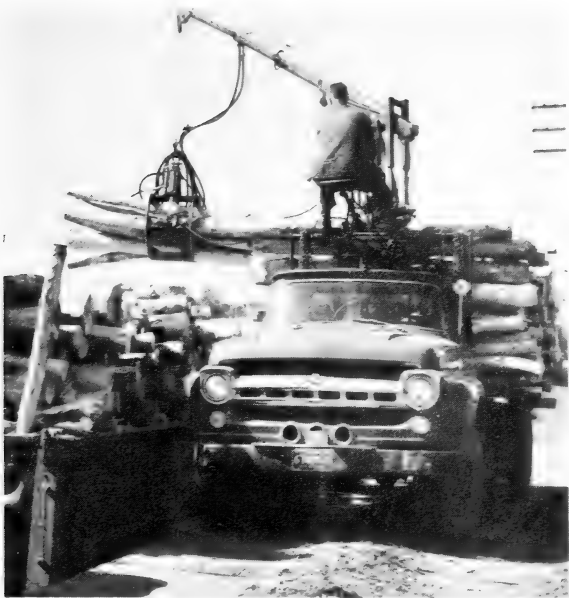
Trucks equipped with mechanical devices facilitate the unloading of logs onto railroad cars. These devices are also used in the loading operation.
