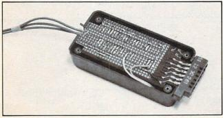
Photo 2: Inside interface, showing bottom of board.
