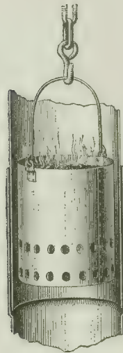
Fig. 306.—Charcoal Fire Pot Within a Pipe.
