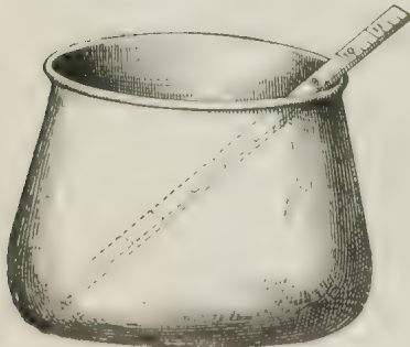
Fig. 164. --Braziers' way of Measuring Saucepans, etc.
