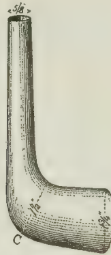
Fig. 82.—Dimensions of Tea-Kettle Spout.
