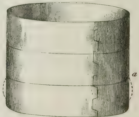
Fig. 165. --Body Marked for Razing.
