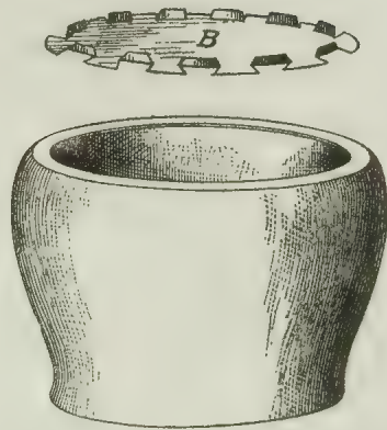
Fig. 167.—Lag Drawn in for Bottom.
