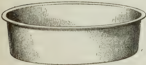
Fig. 211.—Pan Turned for Wire.
