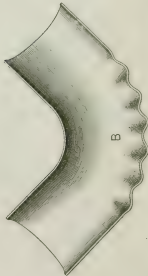
Fig. 318.B.—Piece with Outer Edge Wrinkled.
