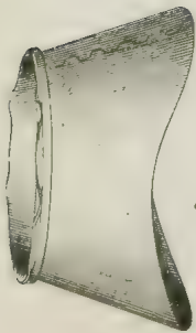
Fig. 414. -- Band Placed on Lower Part While Being Worked.
