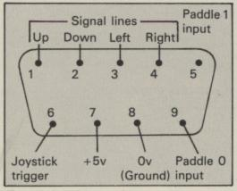
Figure 1: Joystick port pin-outs
