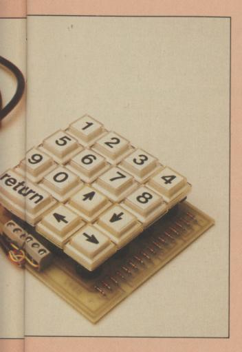
control more than one line without electronic help. But a simple diode matrix is all that's needed — and the circuit shown in Figure II will work perfectly well. When any of the keys is pressed, it connects one or more signal lines via the diodes to Ov, while the other lines remain held at 5v by circuitry inside the computer.
