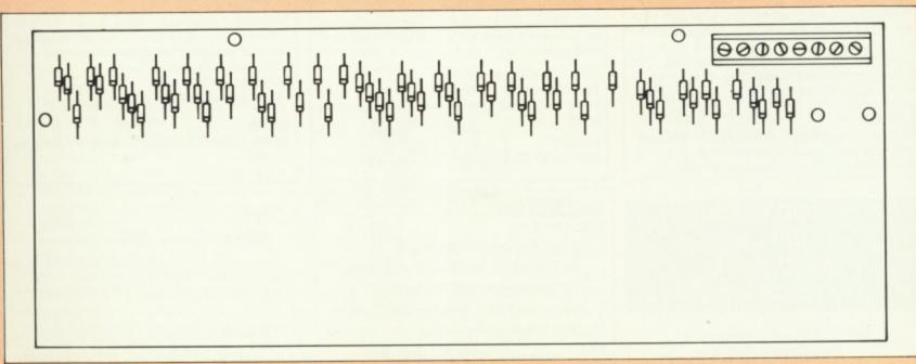
Figure II: Layout showing the position of the diodes on the reverse of the PCB
