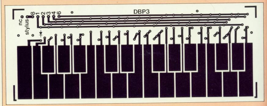
Figure 1: PCB foil pattern
