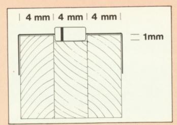
Figure III: The bending jig
