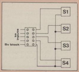
Figure VI: Improved switching network
