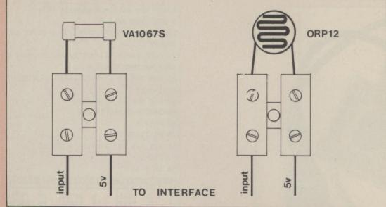
Figure VII: Temperature and light sensor units
