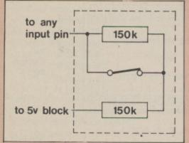
Figure V: A tamper-proof switch for use on doors and windows
