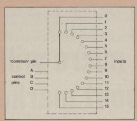
Figure 1: Theory of switch operation
