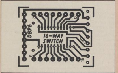
Figure II: PCB Foil pattern
