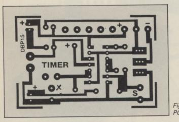
Figure II: The PCB (full size)
