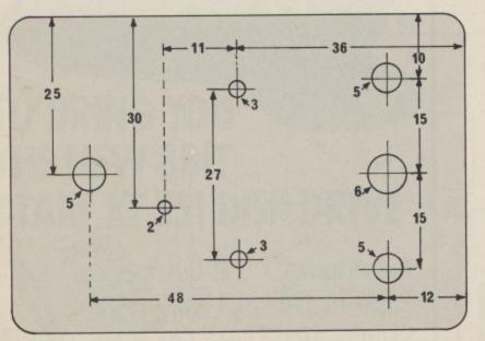
Figure IV: The position of the holes in the case top
