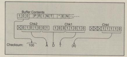
Figure 1: Calculating the checksum digits
