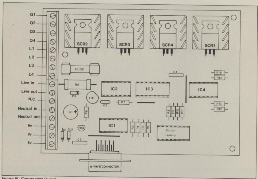
Figure III: Component layout
