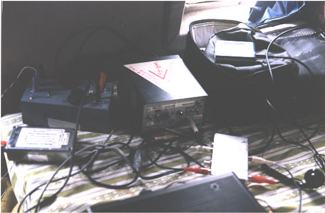
Inside van view of the two VLF receivers, patch-box and cords, and Sony mini-disc recorder in upper right corner
