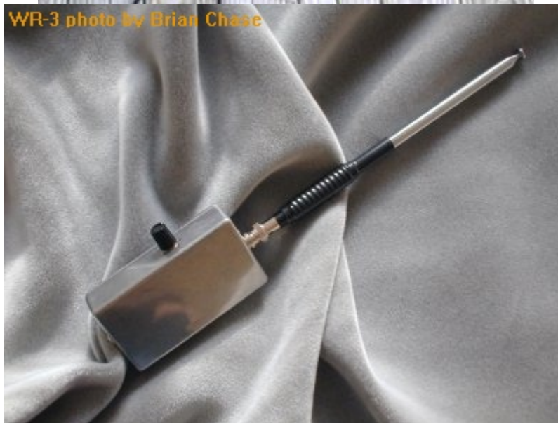
May 2001 photo of the WR-3 shown with Superstick II BNC-base telescoping whip antenna
