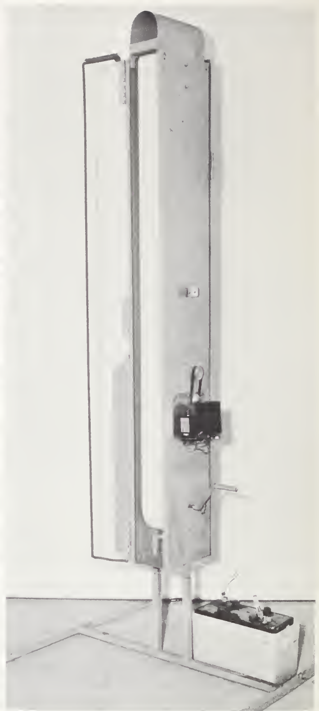
Figure 2.—Insect trap with transparent door open, showing electrical components.
