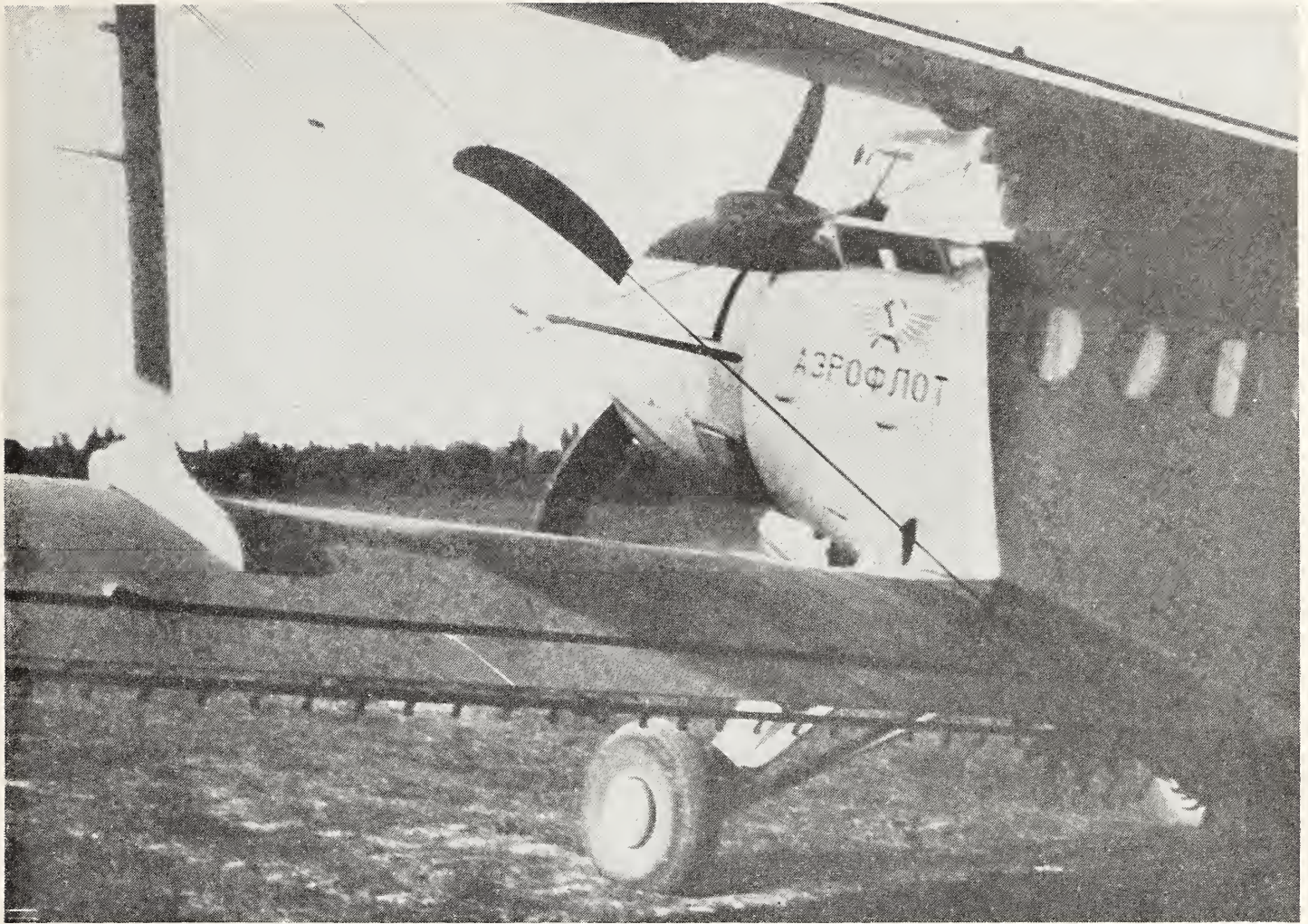
FIGURE 2.—Spray boom of airplane used for spraying cotton in Uzbekistan.
