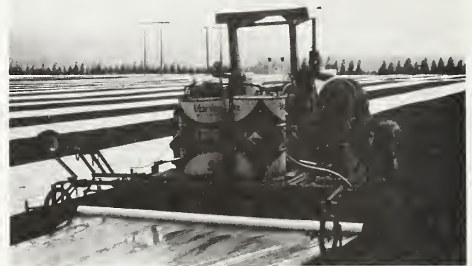
Figure 2 - Strip fumigation consists of treating separate strips of the field, and then returning to fumigate the untreated sections.
