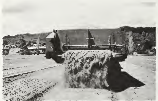
Figure 2.--A commercially-available manure spreader was modified with a mesh conveyor chain, a smooth plastic deck, and an adjustable tailgate (A); these modifications, plus the proper tractor speed, apply a consistent, uniform depth of sawdust mulch over the sown seedbed (B).
