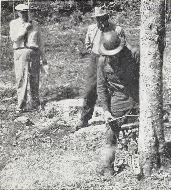
FIGURE 15.—Druzhba gasoline chain saw in operation, showing the "stand-up" frame.
