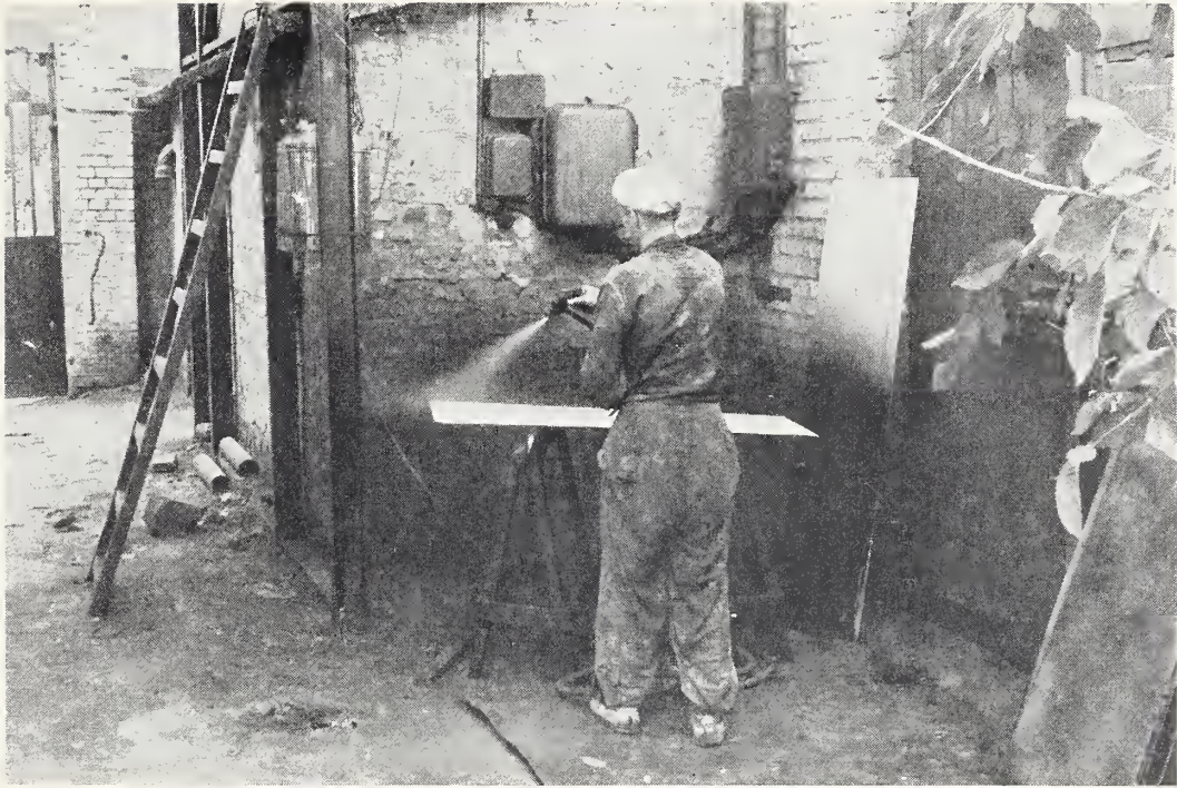
FIGURE 33.—Spraying stain outdoors at the Bozhenko Furniture Plant in Kiev.
