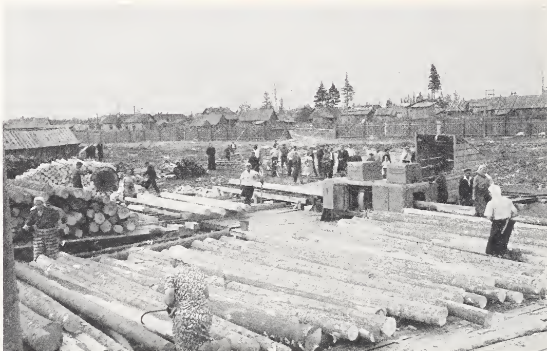
FIGURE 38.—A pulpwod barker of the cambium-shear type at the Shoujsko-Vidanski lower yard. With the exception of men operating the barker and the cut-off saw, all manual labor is performed by women.
