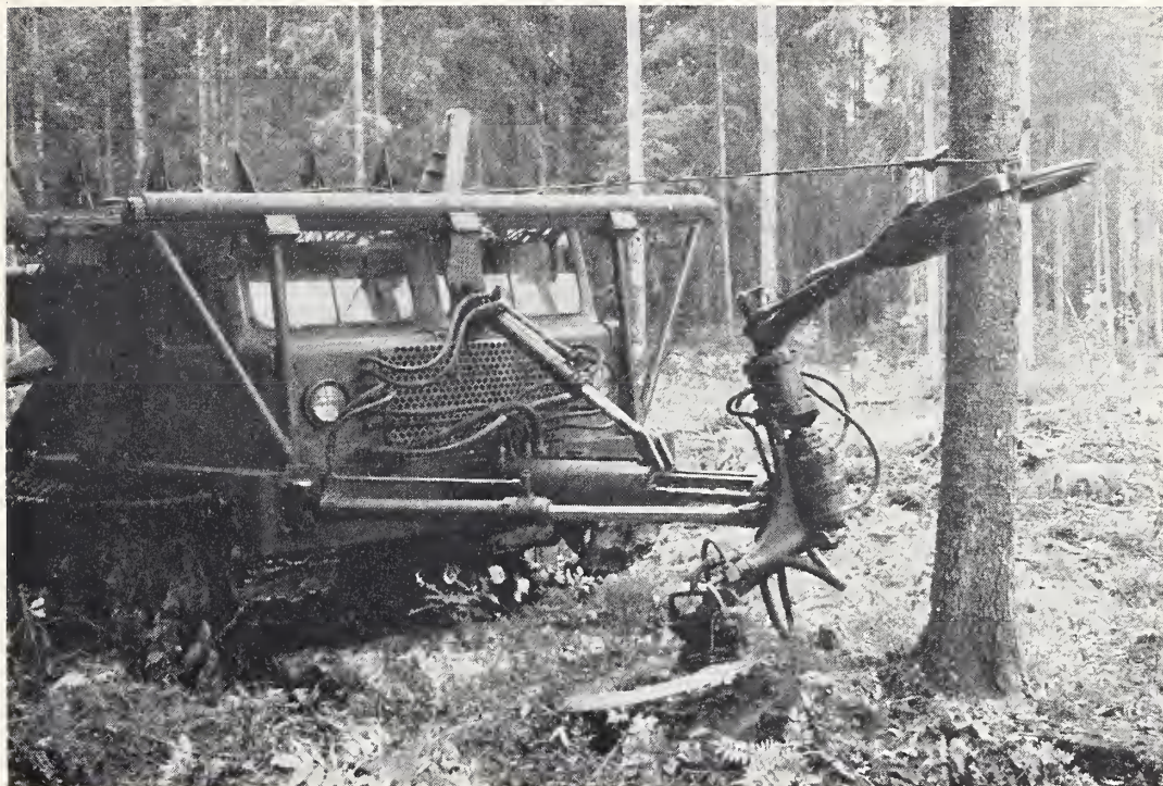
FIGURE 19.—Experimental tree harvesting machine. This is a TDT-90 crawler tractor with 30-inch hydraulic-powered circular saw, steel knee-action claw to grasp tree about 8 feet above the ground, and rear-end winch to pull tree over and bind it to the top of the tractor.
