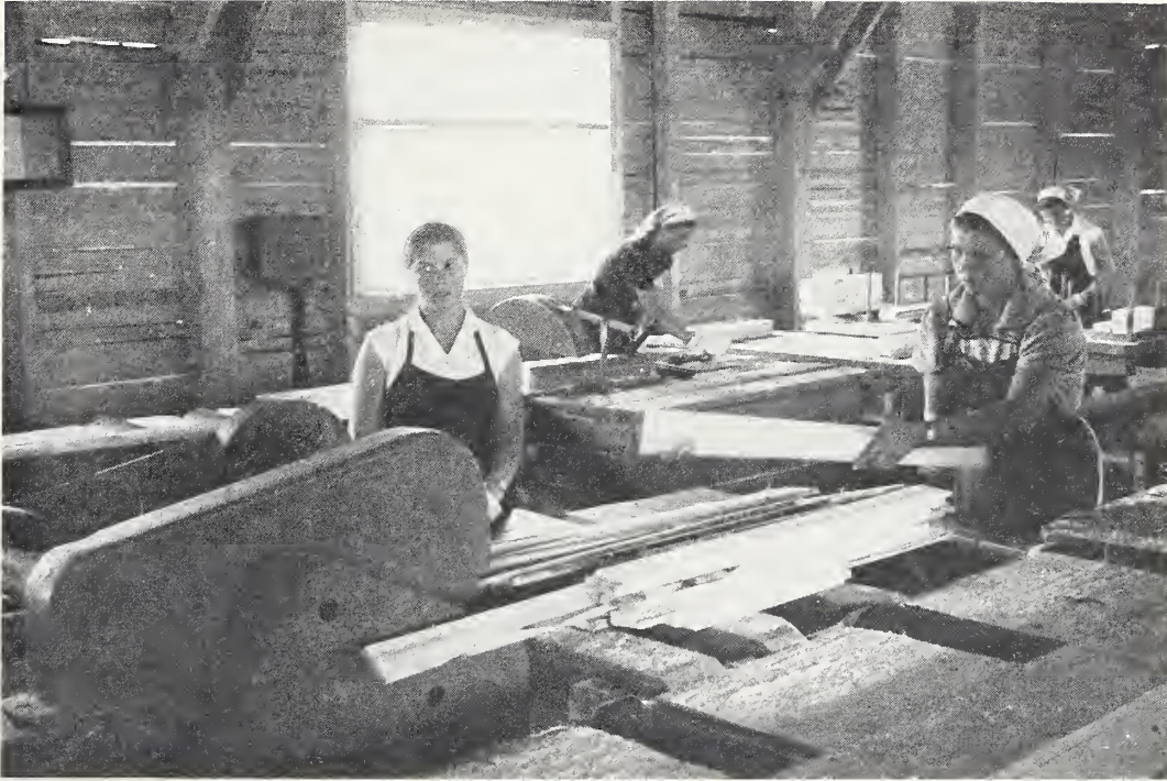
FIGURE 36.—Box shook mill at Krestzy. Some of the low-grade aspen logs, formerly cut into firewood, are now converted into box shook.
