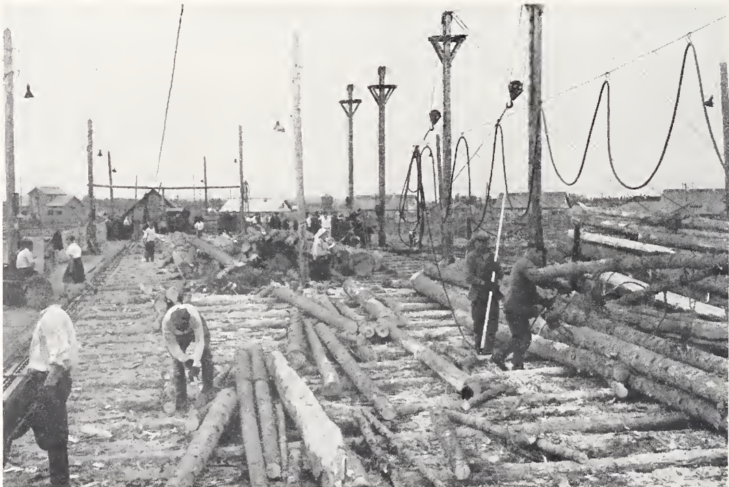
FIGURE 26.—General view of the lower yard at the Shoujsko-Vidanski operation. Electric chain saws are used for bucking logs.
