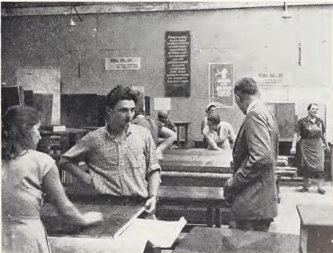
FIGURE 34.—Hand rubbing and polishing of veneered table tops in the finishing room at the Bozhenko Furniture Plant.
