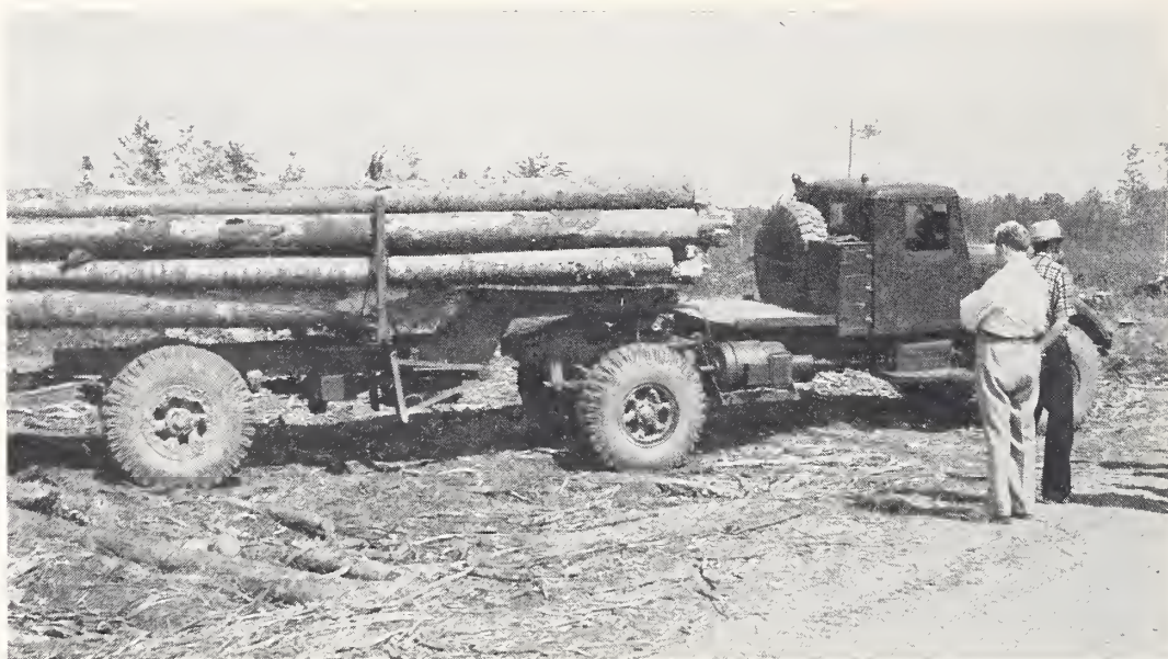
FIGURE 22.—A roadless logging truck with electric-driven bogey. The electric generator driven by the truck engine can be seen behind cab.
