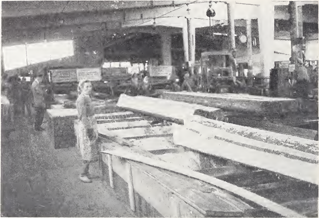
FIGURE 30.—Cants developed by the headsaws. These are resawed into the final products by gang mills, one of which is shown in the right upper corner of the photograph. Stalingrad.
