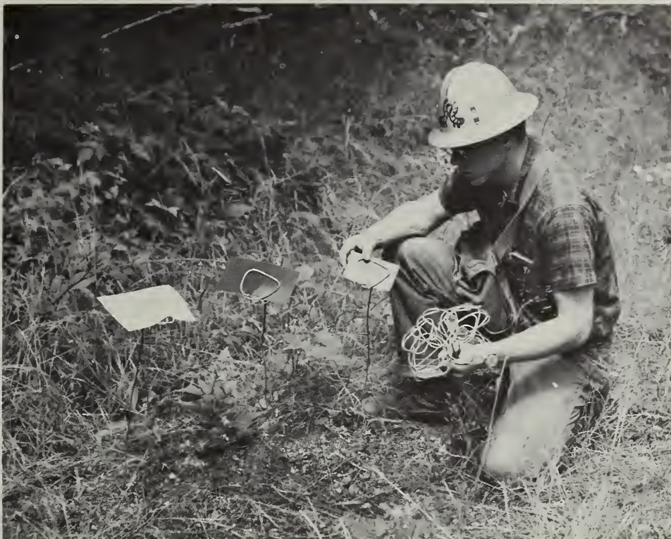
Figure 2.--Placing spray cards and filter paper in wire holders. Left to right, 5x7-inch filter paper, 5x7-inch black card, and 4x5-inch oil-sensitive card.
