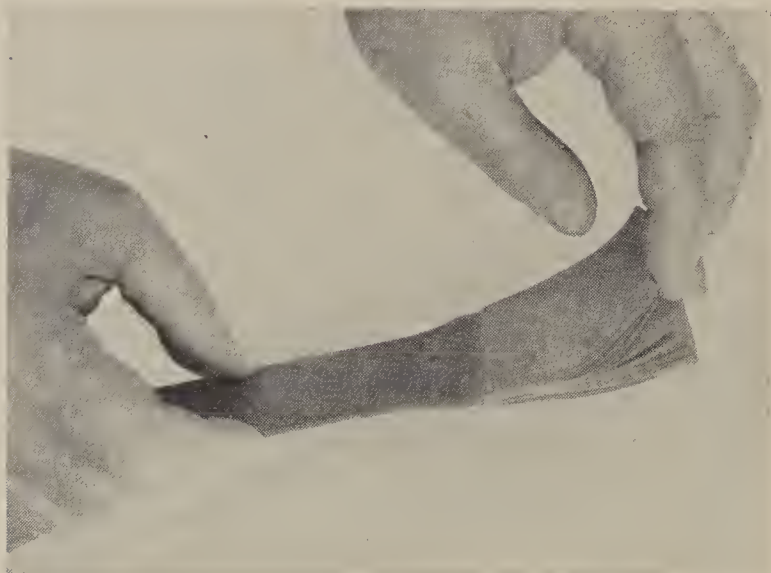
This papreg specimen has been left uncompressed at one end to show the sheets of resin-treated paper of which it consists.
