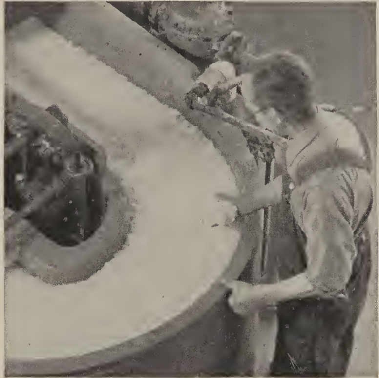
Pulps are further refined in the beater.
