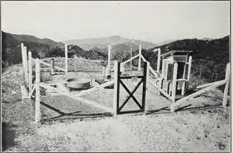
Climatic Station at 4350 feet altitude equipped for measurement of environmental factors of air and soil.
