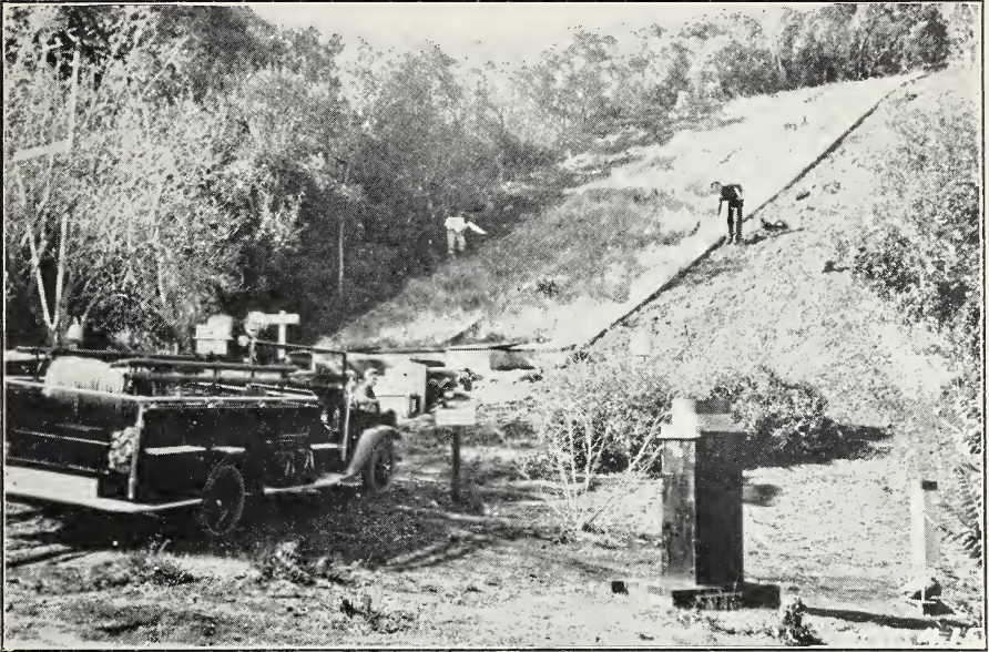
San Dimas Run-off and Erosion Plots. Annually denuded plots (1/40th acre each) about to be reburned. A pair of plots identical in size are located in original brush cover at left. The rainfall and run-off are measured continuously through tipping bucket devices and recorded electrically on a strip chart. Eroded material is collected in a trough and silt trap at the lower end of each plot.
