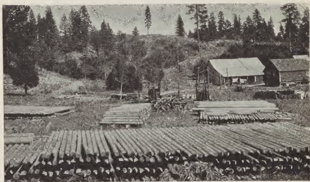
Forest Service fence posts and telephone poles treated with preservative to increase durability. Payette National Forest
