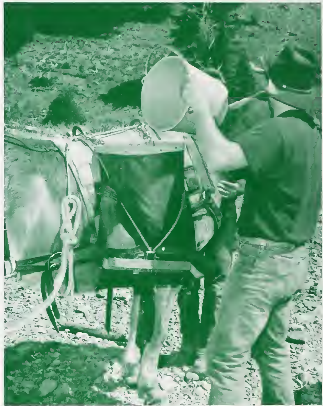
Figure 2.—This design is similar to the first, but has riveted seams and truck tarp fabric. Bags were filled one bucket at a time. Gloves should have been worn.
