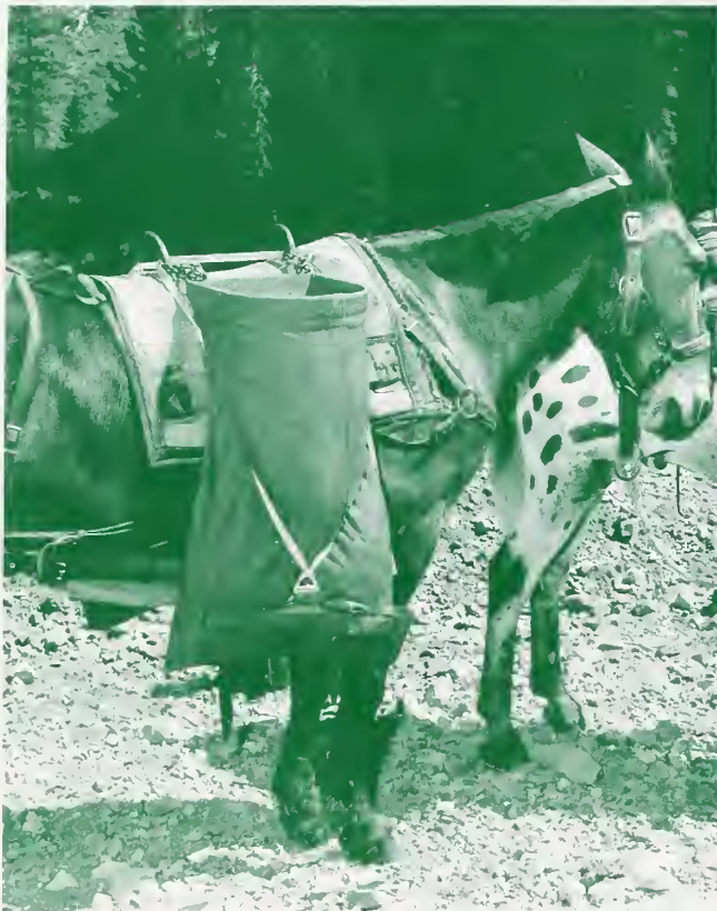
Figure 1.—Gravel bag design features sewn seams around a steel hoop. Release strap was changed slightly in final design.
