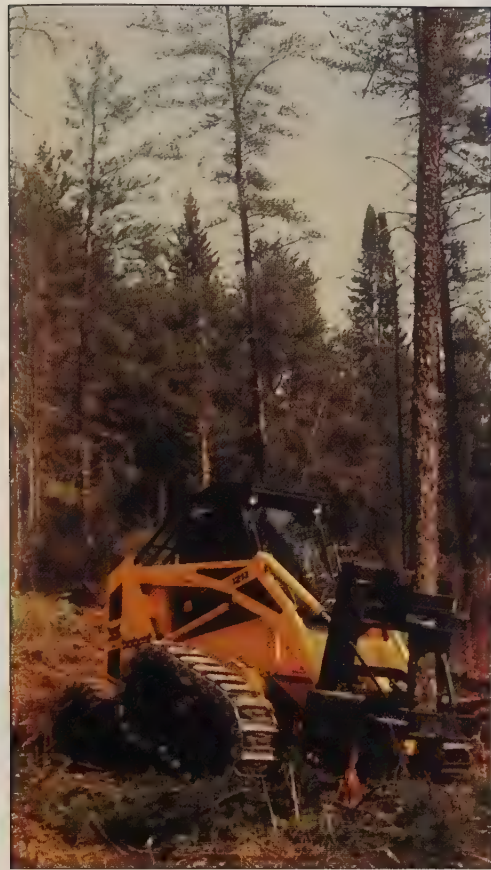
▲ This smaller feller/buncher uses a track system over rubber tires for versatility.
