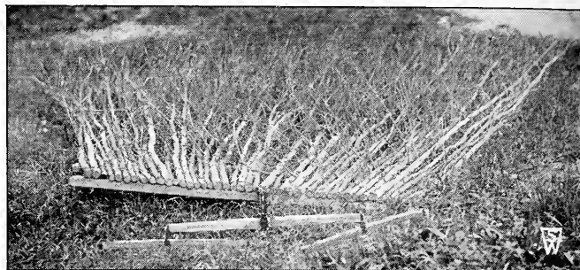
A type of bush harrow as improvised on a New Jersey golf course. Birch branches are used
