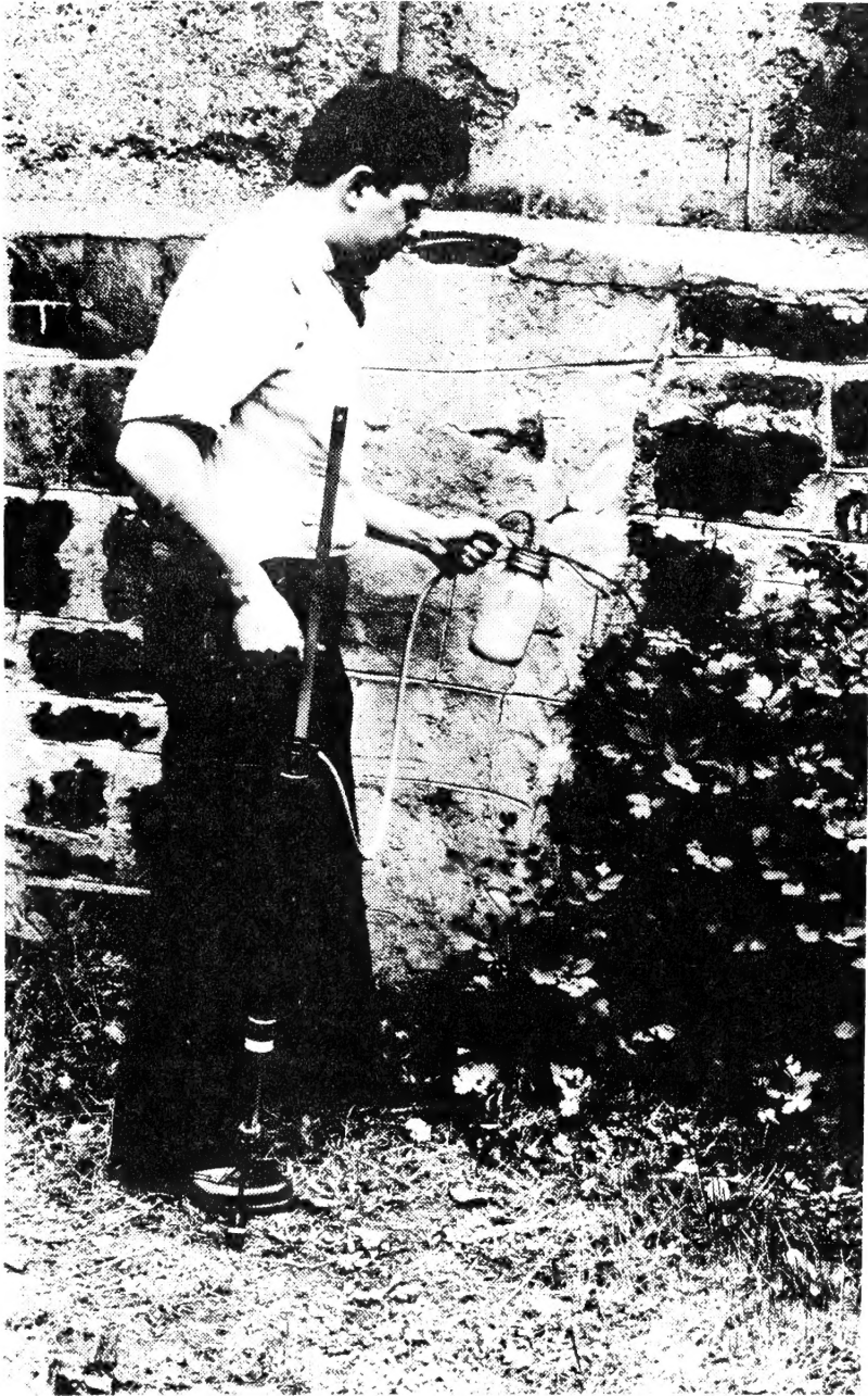
Figure 1.—Equipment in operation. The operator stands with one foot on the foot brace while pumping air through the dust gun.
