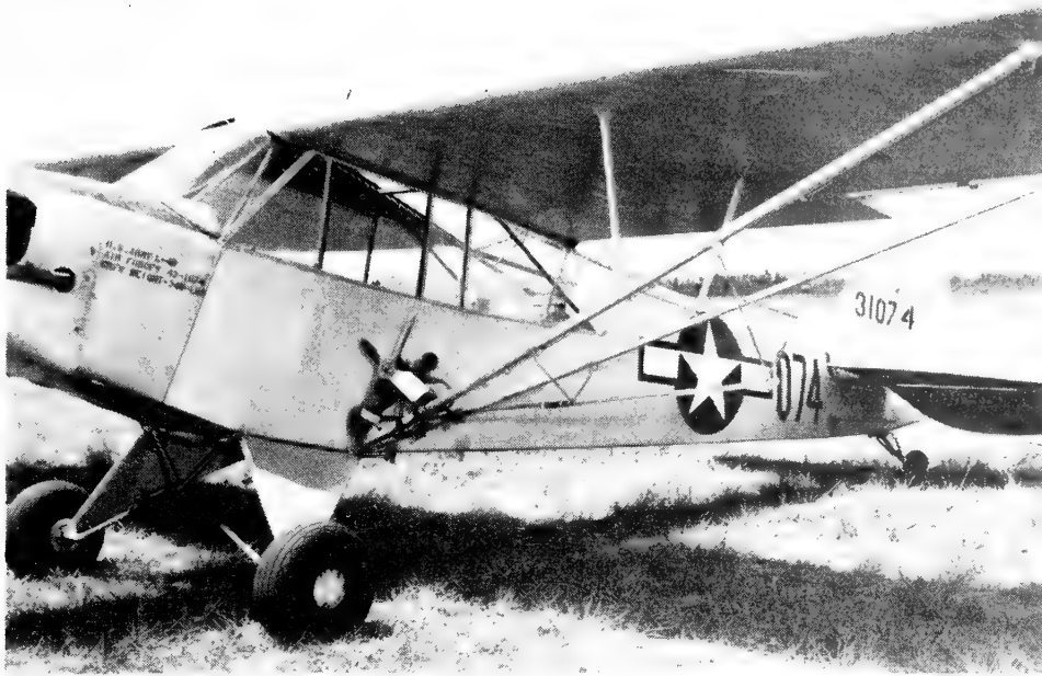
Figure 5.--L-4 series airplane equipped with breaker-bar spray equipment. (Photo by AAFCTR, Orlando, Fla.)
