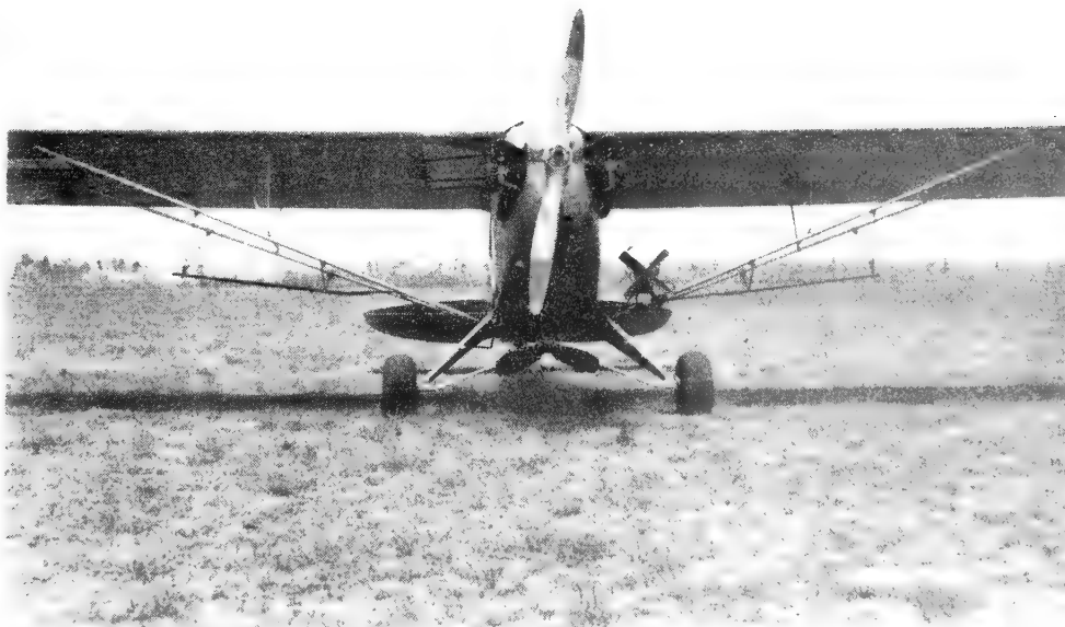
Figure 4.--Breaker-bar spray equipment mounted on L-4 series airplane. (Photo by AAFCTR, Orlando, Fla.)
