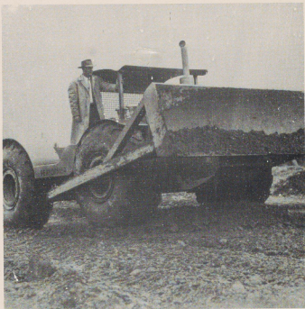
Fig. 1.--"Performer" yarding unit, showing bulldozer.
