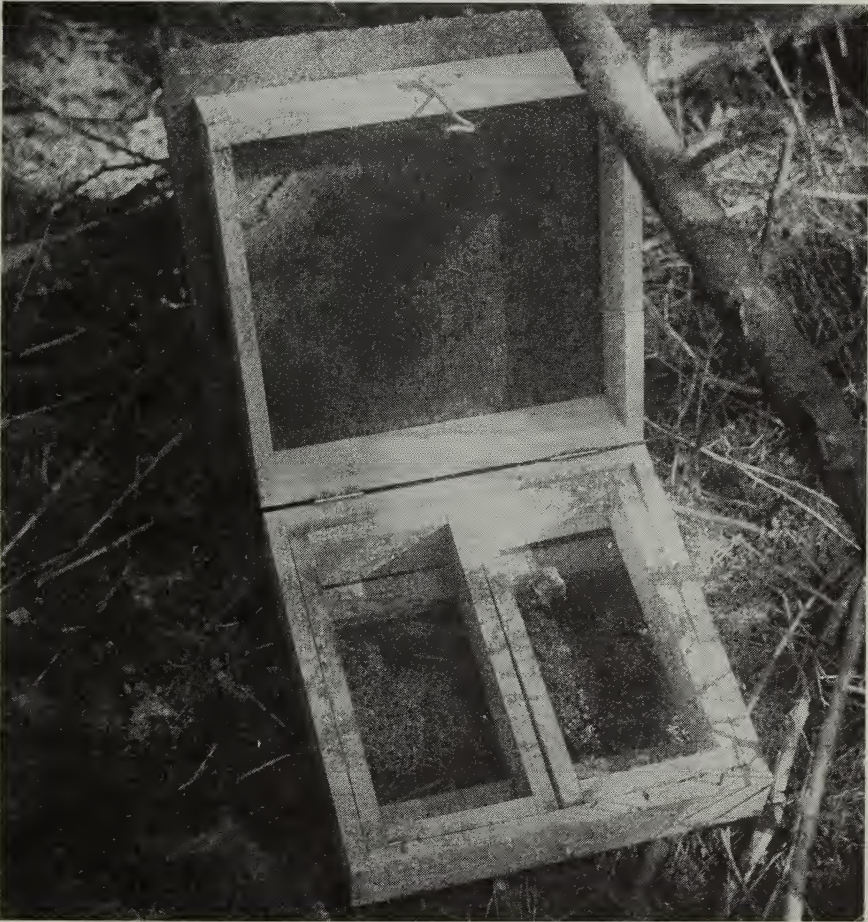
Figure 1. — Feeder in place, with top open to show trays and seed. One tray contained balsam fir seed, the other spruce seed. .
